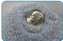
Optical media particles: <1.5mm 2 , nearly as fine as salt
